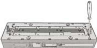
(Optionally take away the IP54-cover by loosening the 4 fixing screws). Now loose the top enclosure at the snap hooks by the help of a corresponding screw driver.
